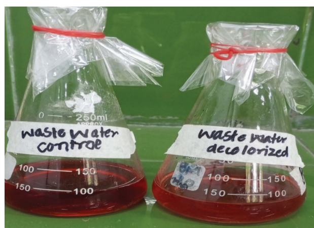
Fig. 3. Flask 1, containing only wastewater, acts as a control, whereas flask 2 contains decolorized wastewater treated with the fungal strain.
