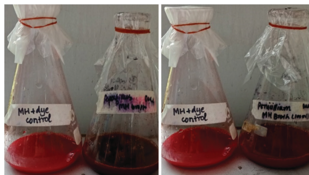
Fig. 1. Color change/degradation of azo dye in the presence of A. niger (left) and P. simplicissimum (right) as compared to the control.
